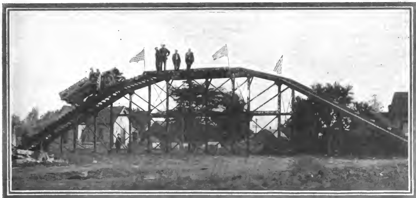
Fifty per cent. gradient over which the Buckeye Manufacturing Company, of Anderson, Ind., tests its Lambert cars
